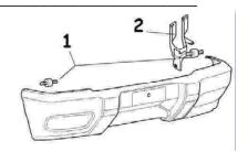
2 Now to fit the Winch Bumper. Some help will be useful at this stage so find 2 strong people to lift the bumper while the third aligns the holes and pushes the bolts through. If fitting a winch, it may be an idea to put it in place now as it may be difficult to do so when all the bolts are tightened.
